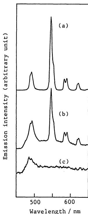
Fig. 2. Fluorescence spectra of TbCl_3 \cdot 6H_2O (a), (1 : 1) mixture of TbCl_3 \cdot 6H_2O and K_3[Fe(CN)_6] (b), and \{Tb[Fe(CN)_6] \cdot 5H_2O\}_x (c) in solid state. Exciting wavelength is 355 nm. Slit widths(nm) of (excitation and emission sides) are (2 and 2). Ordinate scales are \times 8 for (a), \times 512 for (b), and \times 1024 for (c). Filters, UV-35 and V-Y47, are used for excitation and emission sides, respectively.
